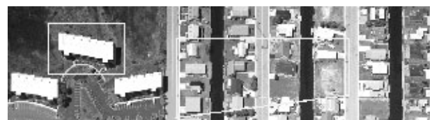
Figure 3: The study site for the experiments reported in this paper is a small area of the Ocean City Test Site, established by ISPRS WGIII/5. The apartment complex (left) has a flat roof but a fairly complicated roof outline. A DEM with 2 m grid spacing was measured on and around the building. Similarly, a DEM was measured in the highlighted part of the residential area.
